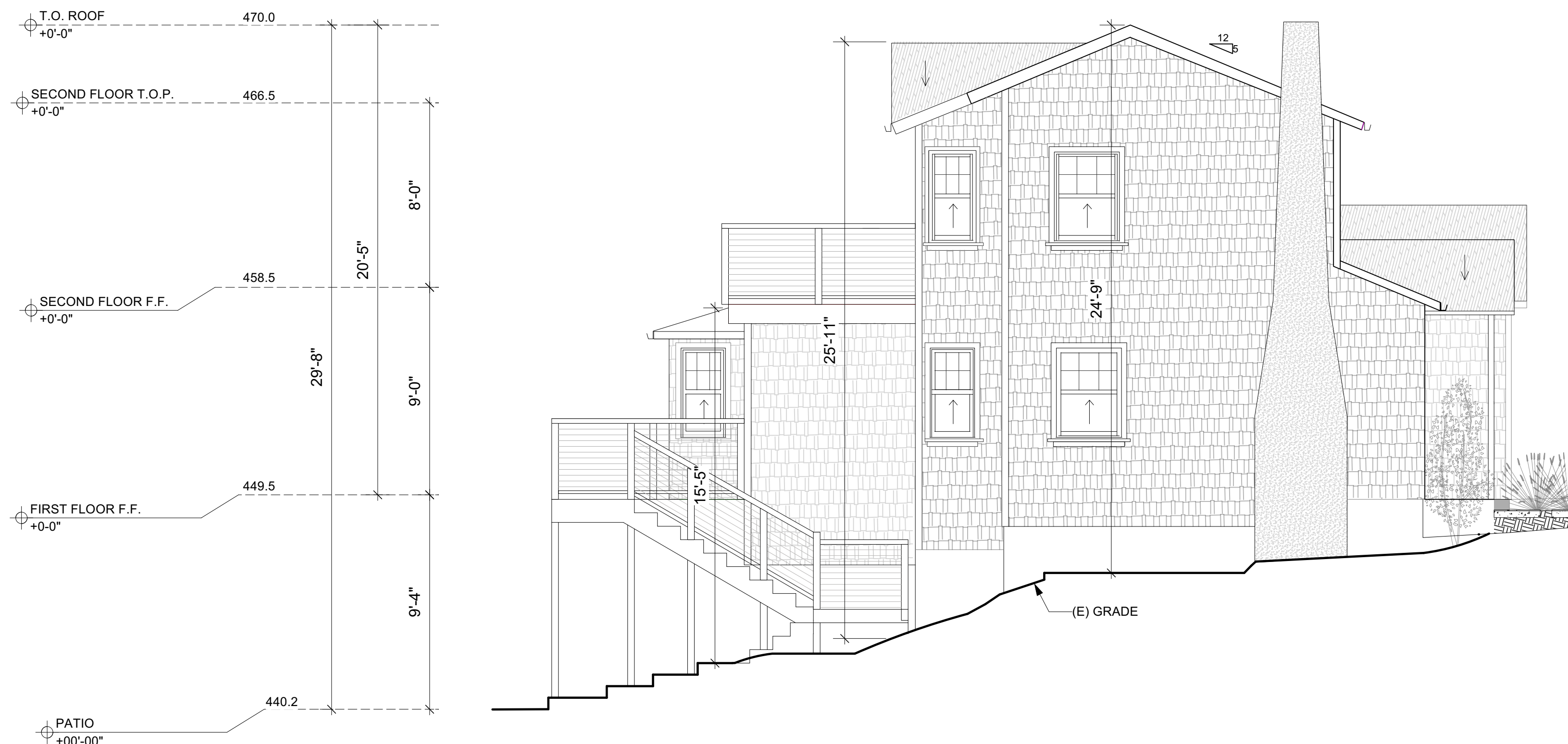
3 EXISTING WEST ELEVATION - NO CHANGE SCALE: 1/4"=1'-0"
