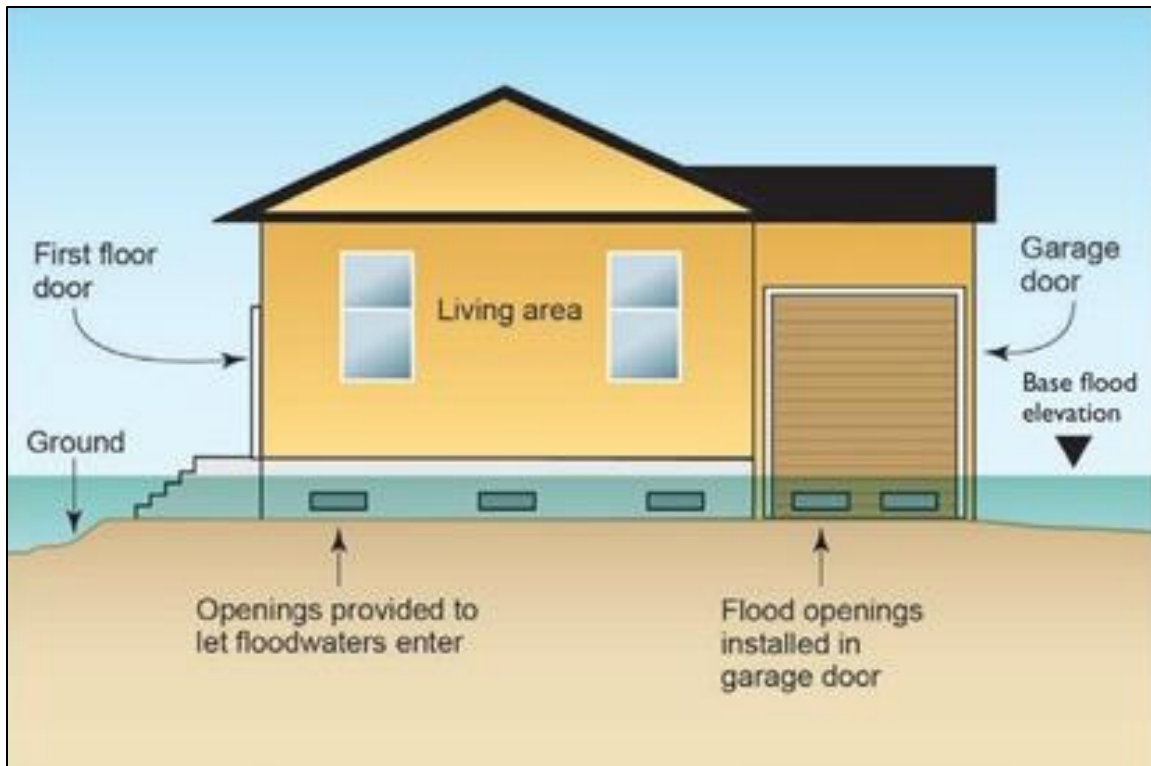
Figure 3. Wet Floodproofing Diagram
