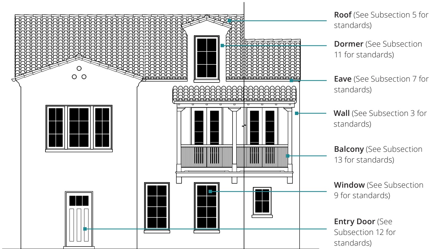
Prototypical Building Elevation
