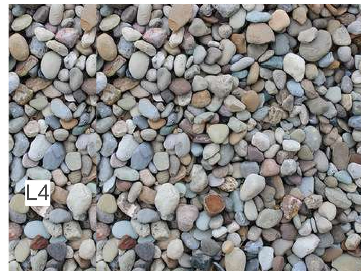
L4 Washed Gravel Also Known As: #4 River Gravel, #4 Round Gravel Size: 1 1/2" to 3/4" Uses: Landscaping, roofs
