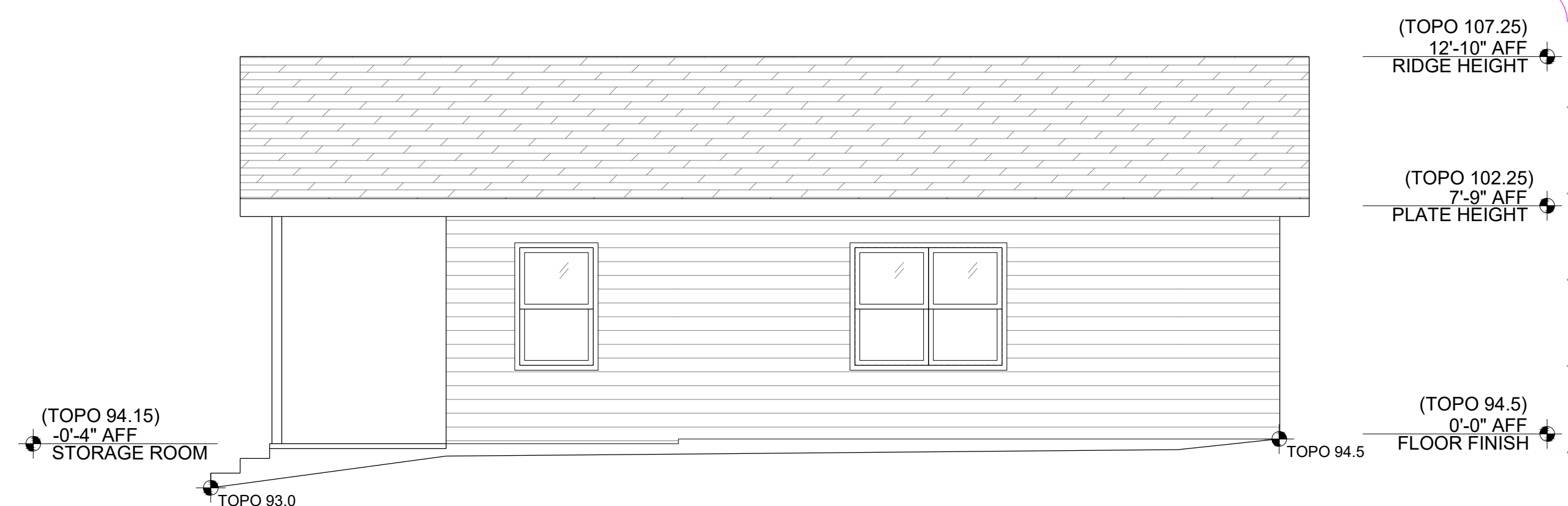
5 EXISTING NORTH ELEVATION - NO CHANGE Ac2.0 SCALE 1/4" = 1'-0"
