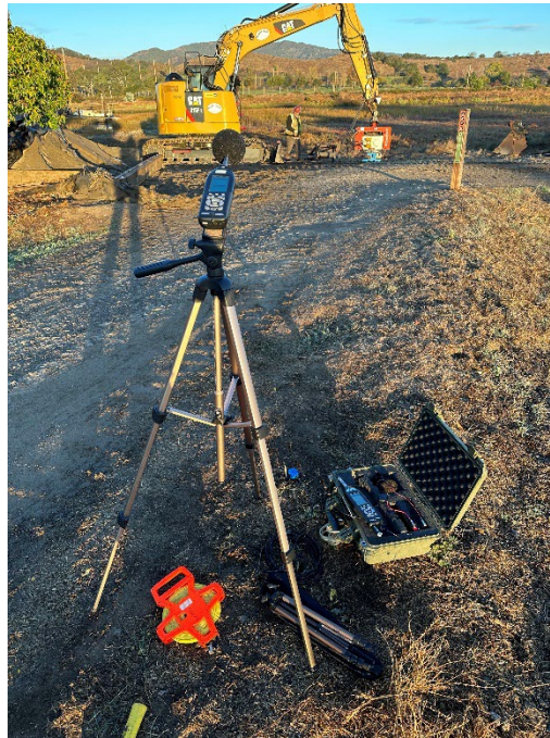
Photo 3: Noise and vibration meters at Site 1.
