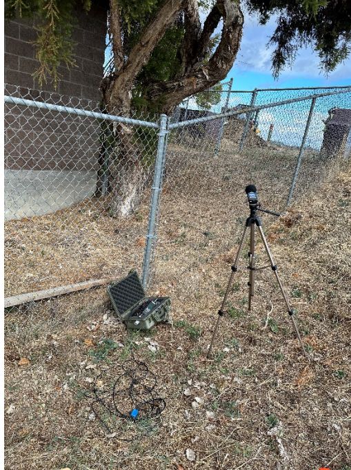
Photo 5: Noise and vibration meters at Site 3.
